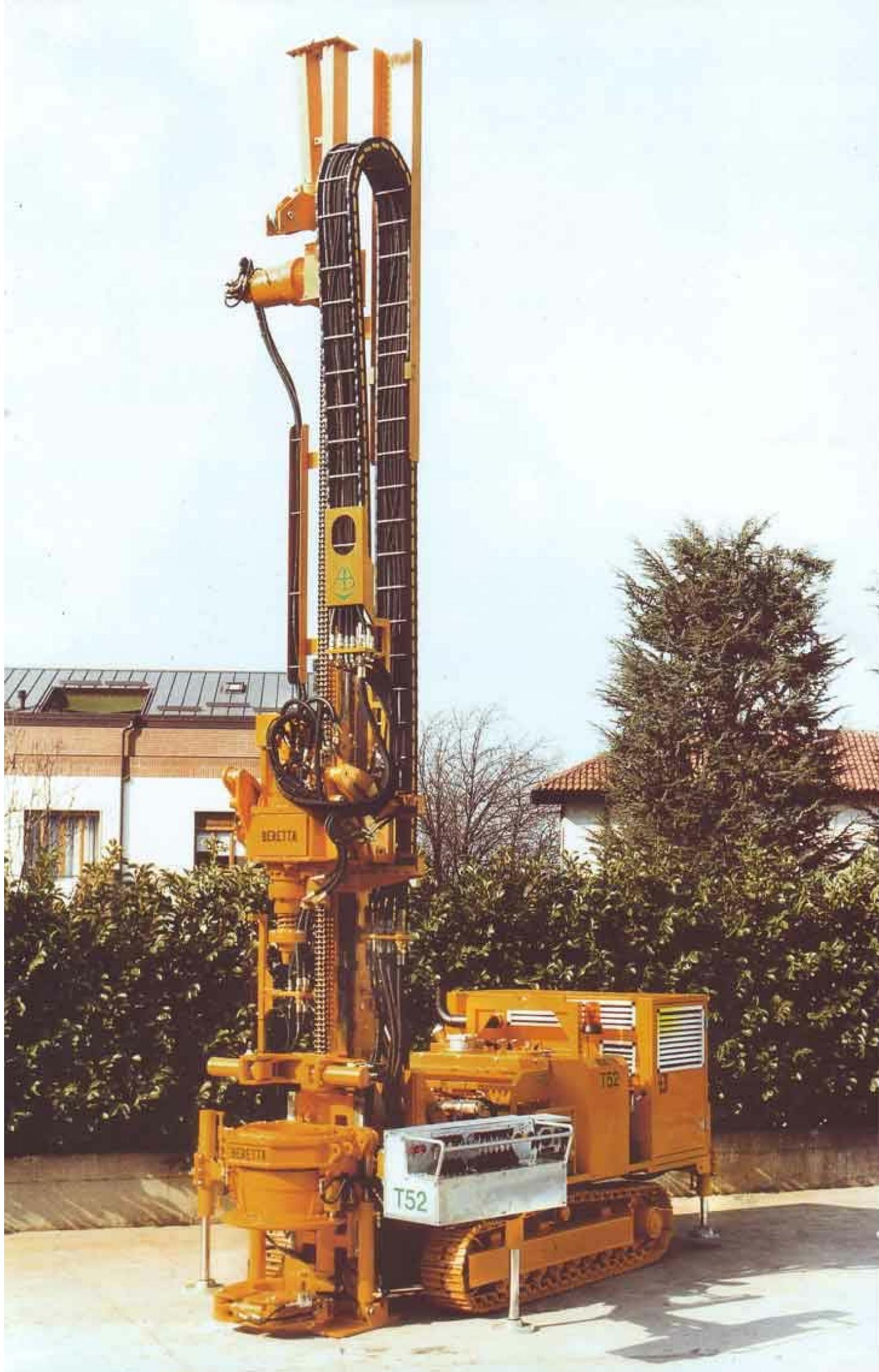
**Perforatrice Idraulica • Hydraulic Drilling**
